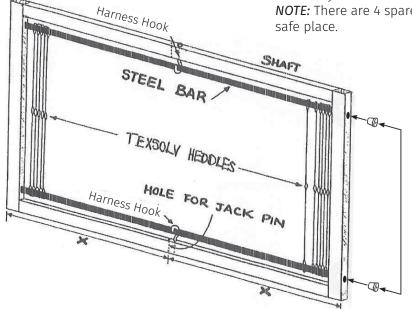
Spread the heddles evenly either side of the Harness Hook and then clip the stainless steel rods over the hooks. The hooks prevent the bars from sagging when being raised or pulling out when the warp is being advanced.
