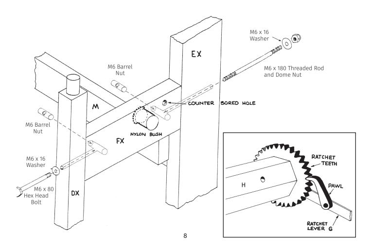
12. Insert the 12 x 1 Pan Head Screw into the inside of the front upright **DX** for a ratchet lever stop. When transporting the loom lift and pull the lever sideways, then let it hang down.
