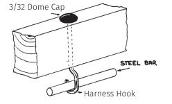
24. Each shaft has holes on both edges of top and bottom rails. The hole for the jack pin is exactly in the centre of the bottom rail to ensure it lifts evenly and is marked with a small hole on the front of the shaft. **Do not use this hole for a hook.**
