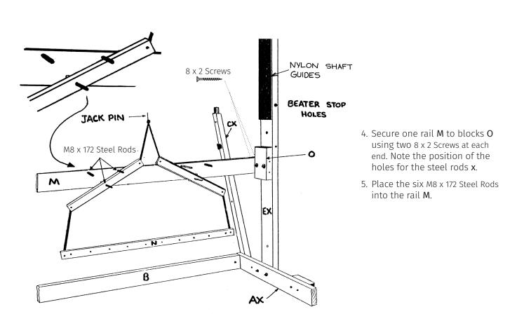
6. Apply a drop of oil onto the two lower steel rods. Then slide 5 x M8 x 25 washers onto the two lower steel rods followed by a lever assembly **N**. Place two washers onto each lower steel rod followed by another lever assembly **N**. Repeat this procedure until all the lever assemblies are in position, finishing with 5 washers.
