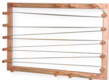
warping frame 11m (37') warp.
